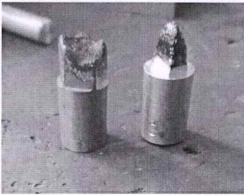
Fig. 4. After machining brass electrodes.
